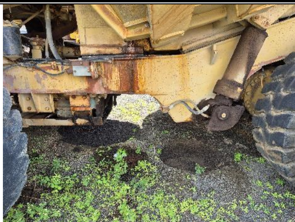
No drip trays – oil spillage
