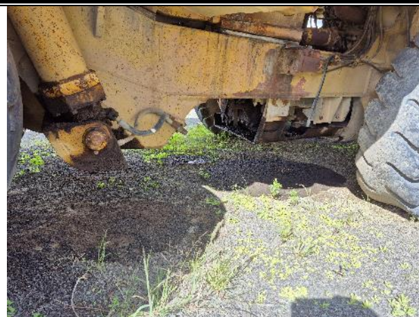
No drip trays – oil spillage
