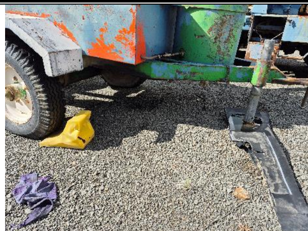
No drip trays – oil spillage
